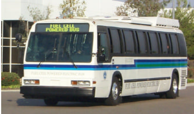
Figure 3a. 40-foot PEMFC Generation 1 Bus
